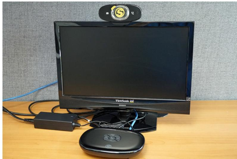
**Figure 5** — nVP2 Main Unit, power supply and camera on video display
