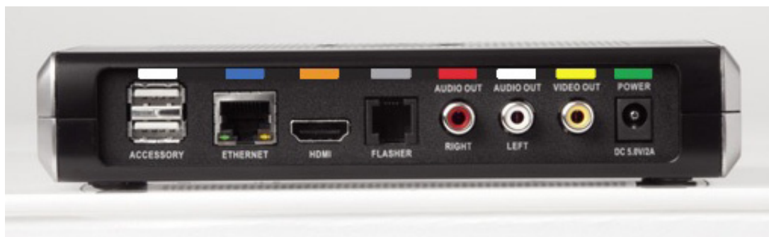
Figure 3: Back panel of ntouch VP Main Unit
