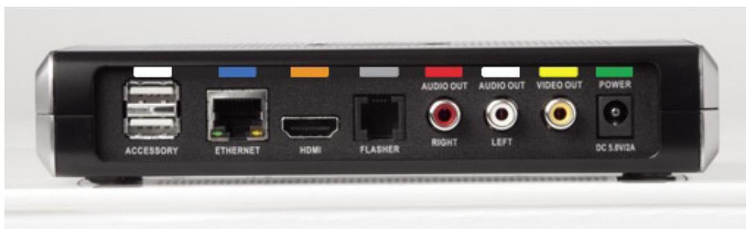
**Figure 3:** Back panel of ntouch VP Main Unit
